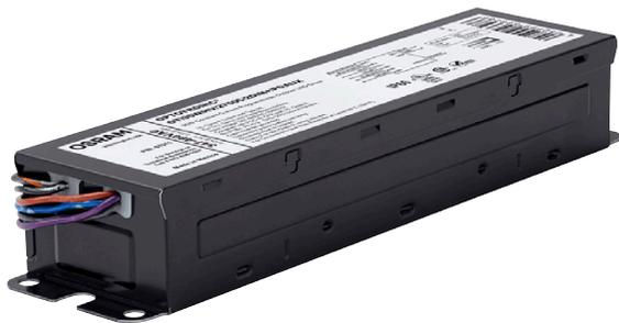
The OPTOTRONIC programmable dimmable family consists of highly efficient, constant current LED drivers for industrial applications. One click programming through the OPTOTRONIC Programmer allows OEMs to configure the output current with 1mA resolution. Also fully customizable by the OEM is an OSRAM proprietary feature called AstroDIM. AstroDIM is autonomous dimming for night time power reduction based on an internal timer that can be set for an entire year.
